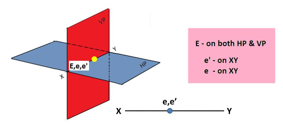
Point on both HP & VP, its Front and Top views on XY
